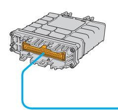
From the incoming values, the EDC control unit calculates the setpoint for injection commencement and sends a corresponding pulse duty factor to commencement of injection valve N108.
