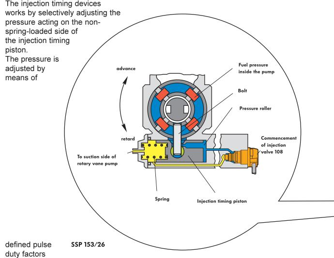
which are used to control commencement of injection valve N108, i.e. an exact point of commencement of fuel injection is assigned to each pulse duty factor.
