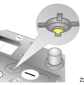
colourless/yellow ... critical acid level, you must top up with distilled water
