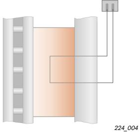
Depending on the model, the "Check brake pad" warning appears on the dash panel insert display or an acoustic warning sounds (Audi).
