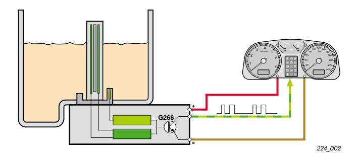
The oil level/oil temperature sender G266 is a thermal oil level sensor. While the engine is running, the engine oil temperature is continuously measured and the engine oil level is calculated. Both parameters are sent via a common pulse-width modulated signal to the dash panel insert.
