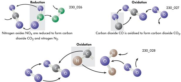
Hydrocarbons HC are oxidised to form carbon dioxide CO<sub>2</sub> and water H<sub>2</sub>O.
