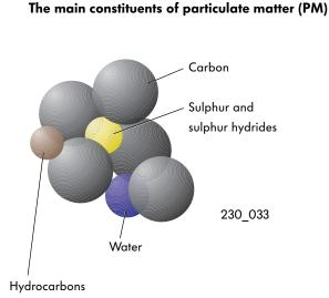
The particulate matter typically emitted by a diesel engine comprises a core and several attached components, of which only the hydrocarbons (HC) are oxidised in the oxidation catalytic converter. The residues of the particulate matter can only be collected by special particulate filters.
