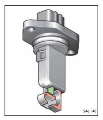
In the variable valve timing system, the signal is used for load-dependent adjustment of the camshaft.
