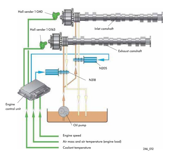
This section goes into more detail about the adjustment of the camshafts. The parts, the design and the operation are the subject of the following pages.
