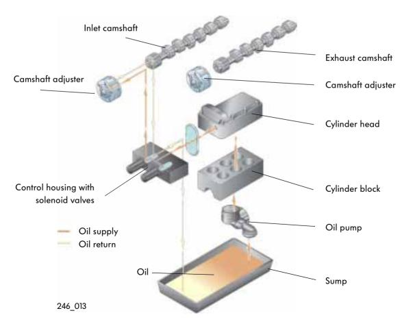
The oil course to the exhaust camshaft is identical with that to the inlet camshaft.
