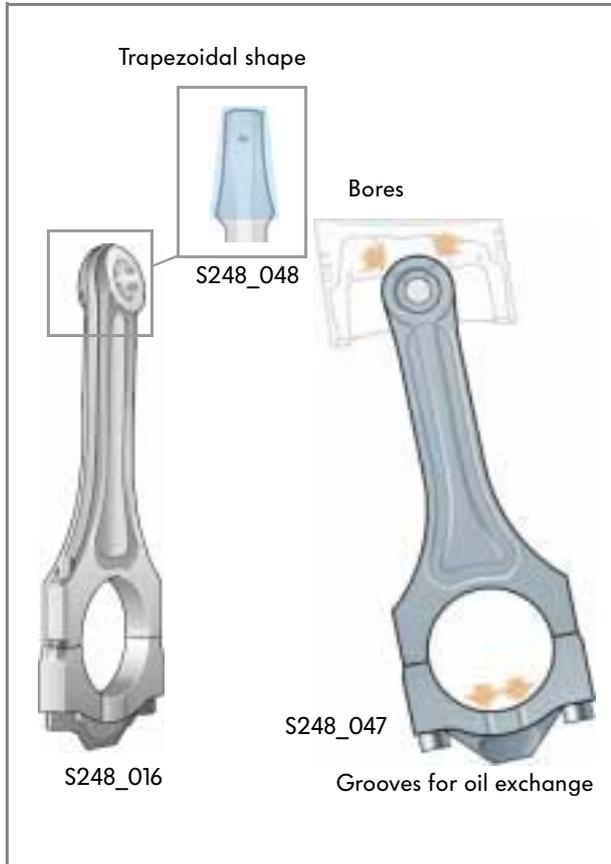
The conrods are made of forged steel and are only 13 mm thick. They are of a trapezoidal construction and are cut during the production process.
