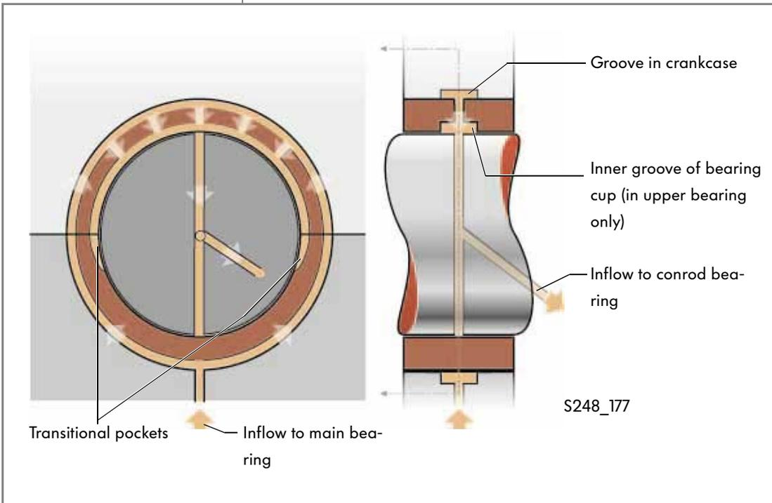
The oil flows from the outer circumferential groove into the inner groove of the upper bearing cup through five bores. The bore ensures that an even oil film forms. Integrated pockets at the transition to the lower bearing cup ensure a steady supply of oil to the conrod bearings via bores in the crankshaft.
