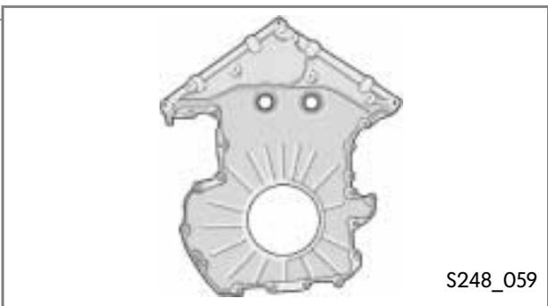
The balancing shaft drive is protected on the belt drive side by a plastic housing cover.
