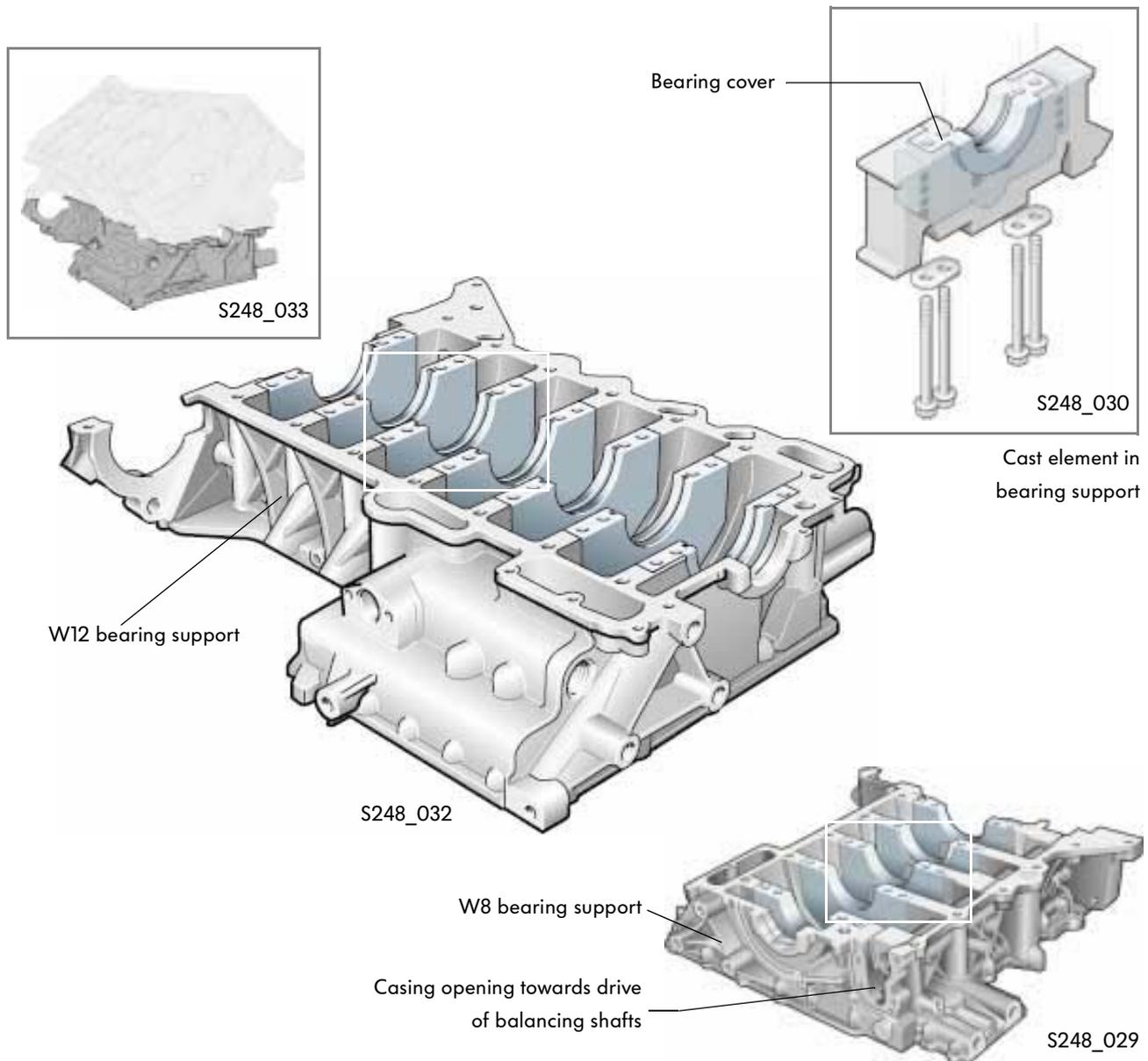
The bearing support is also made of aluminium. It serves as a frame structure for the lower crankshaft bearing covers. These bearing covers are made of grey cast iron and are also embedded when the bearing support is cast.
