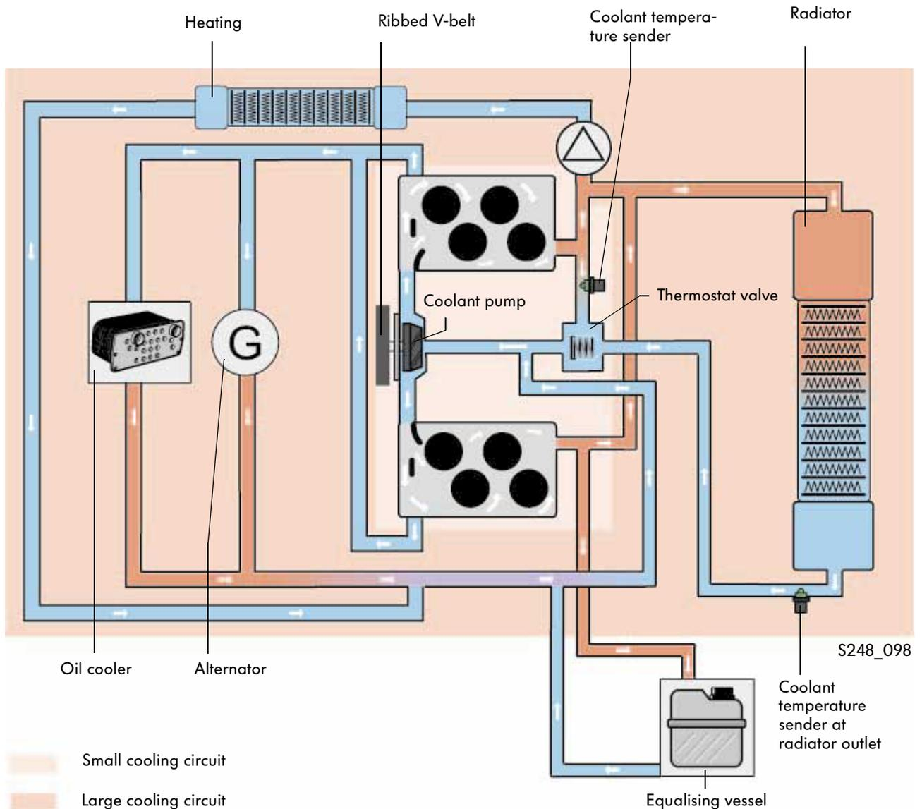
**Coolant circuit of W12 engine**
