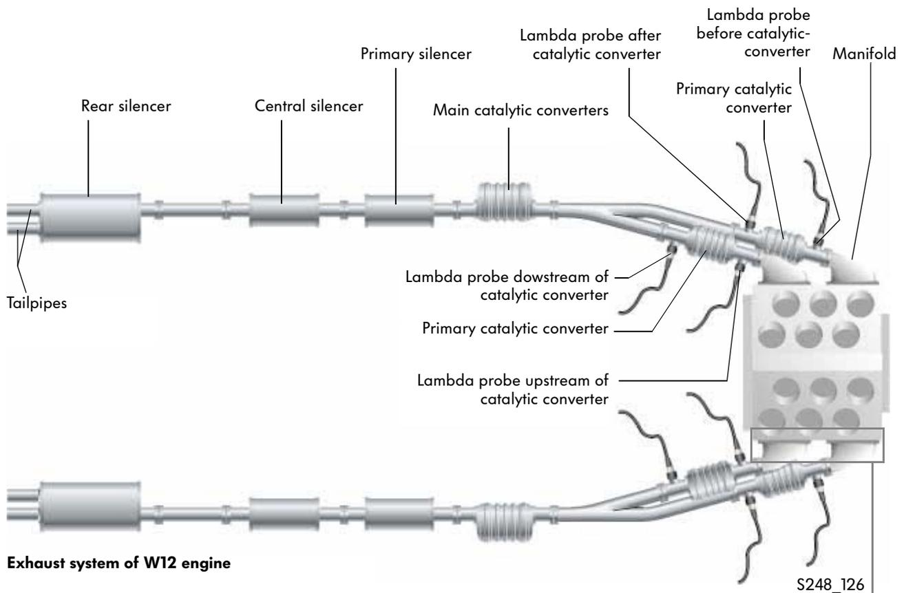
**Exhaust system of W12 engine**
