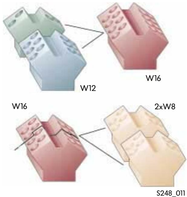
A W16 engine is obtained by joining two cylinders to each cylinder bank of a W12 engine. Splitting the W16 in the middle leaves two W8 engines. A W10 engine consisting of two VR5 engines is also a possibility. This covers the complete range of W engines.
