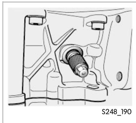
Insert camshaft rule for aligning the camshafts.
