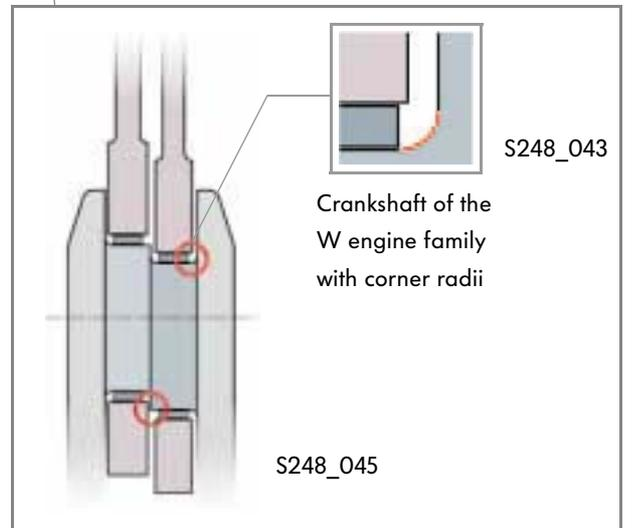
The conrod journals are arranged in pairs and in accordance with the crankshaft throw. When the conrods are installed, the bearing cups must not contact the radii or the edge between the two conrod faces (use tool).
