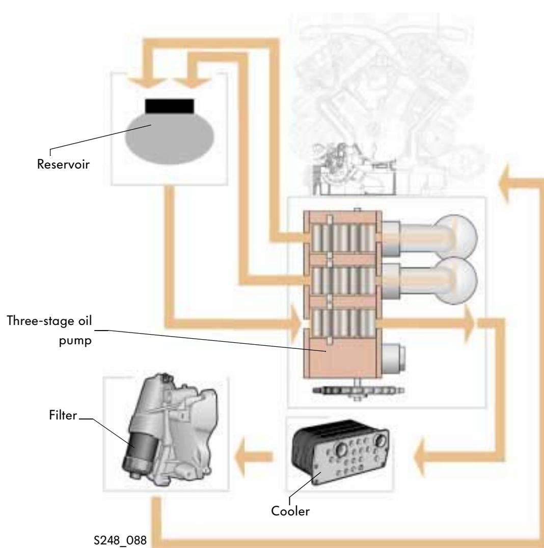
In the case of the dry-sump lubrication system, the entire oil supply is retained in an additional, external reservoir, and not in the oil sump.
