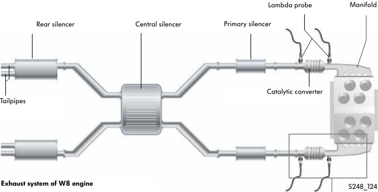
Exhaust system of W8 engine
