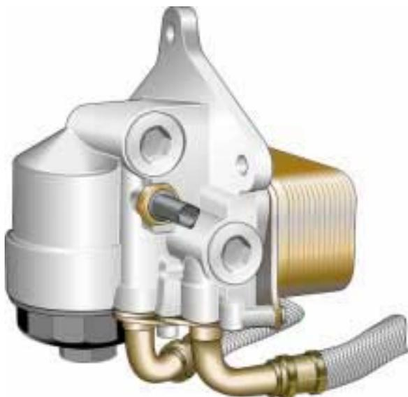
Oil filter/cooler module of the W8
