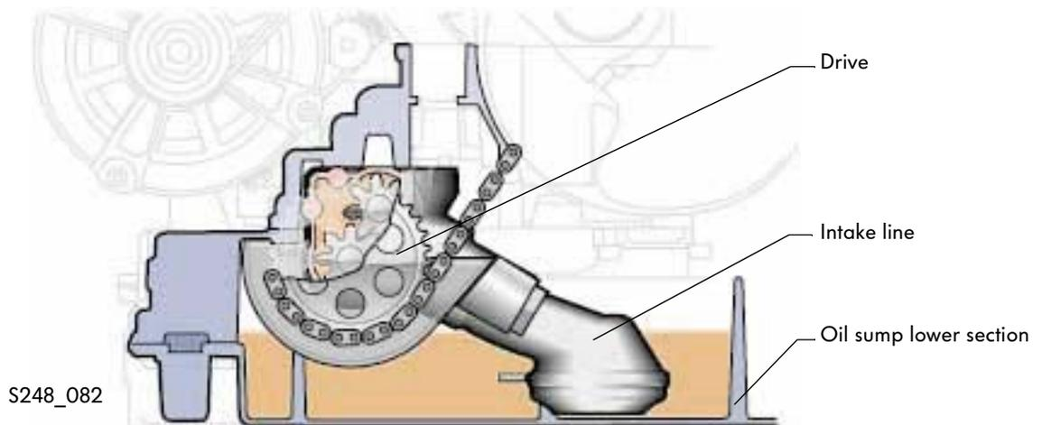
The oil is extracted from the sump by the oil pump via the intake line, and pumped into the oil circuit.
