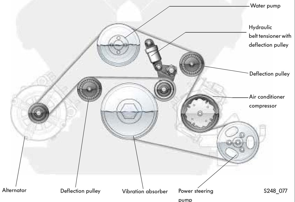
In the W12 engine, the hydraulic belt tensioner and deflection pulley are fixed to the air conditioner compressor bracket.
