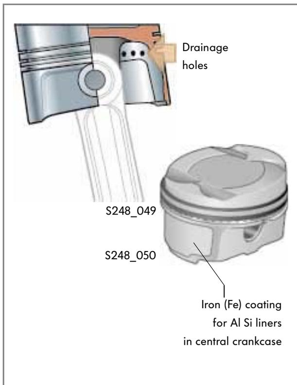
The pistons are made of an aluminium-silicon (Al Si) alloy. The recess in the piston surface is very shallow as the cylinder head takes up most of the combustion chamber volume. The inclined piston surface is necessary because of the V-position adopted by the pistons.
