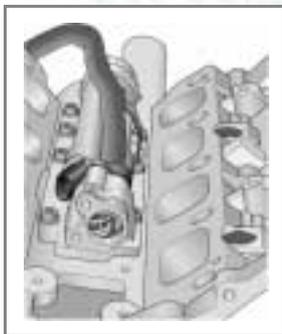
By electrically activating the thermostat valve, it is possible to control the switching point and coolant temperature. Characteristic maps are stored in the engine control unit. They make it possible for the engine to reach the desired temperature in accordance with the engine's operating requirements.
