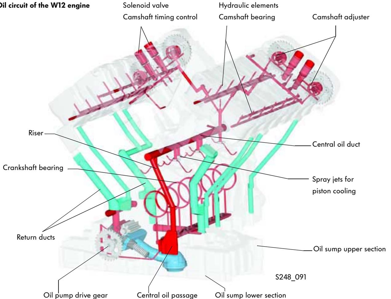
**Schematic diagram of the oil circuit of the W engines**
