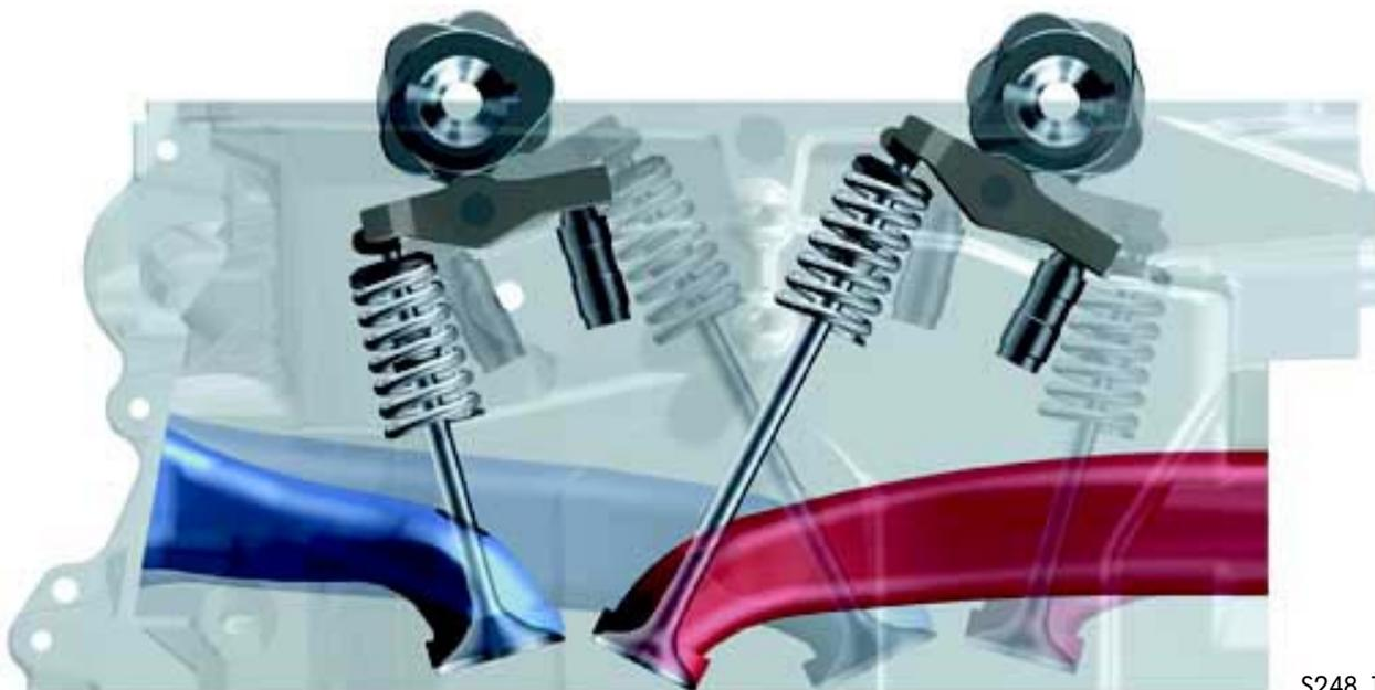
Due to the cylinder arrangement, short and long valves as well as short and long inlet and exhaust ports alternate with one another.
