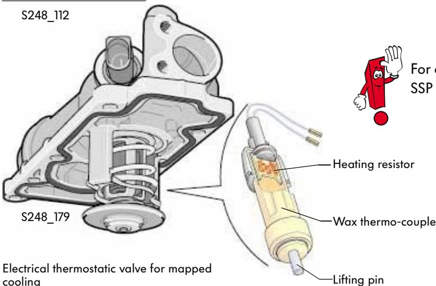
Electrical thermostatic valve for mapped cooling
