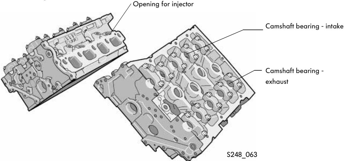
Each of the cylinder heads in the two W engines has an intake camshaft and an exhaust camshaft with camshaft adjusters attached to their end faces.
