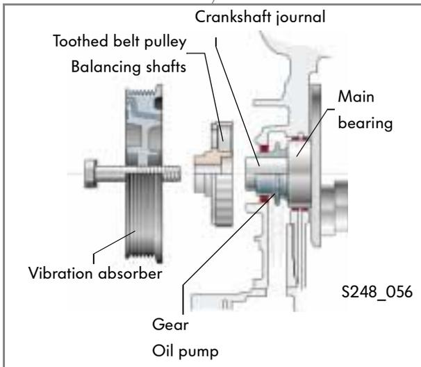
The drive gear of the oil pump, together with the toothed belt pulley for the balancing shafts (on the W8 engine only), is pressed against the outer main bearing and fixed in place by the vibration absorber.
