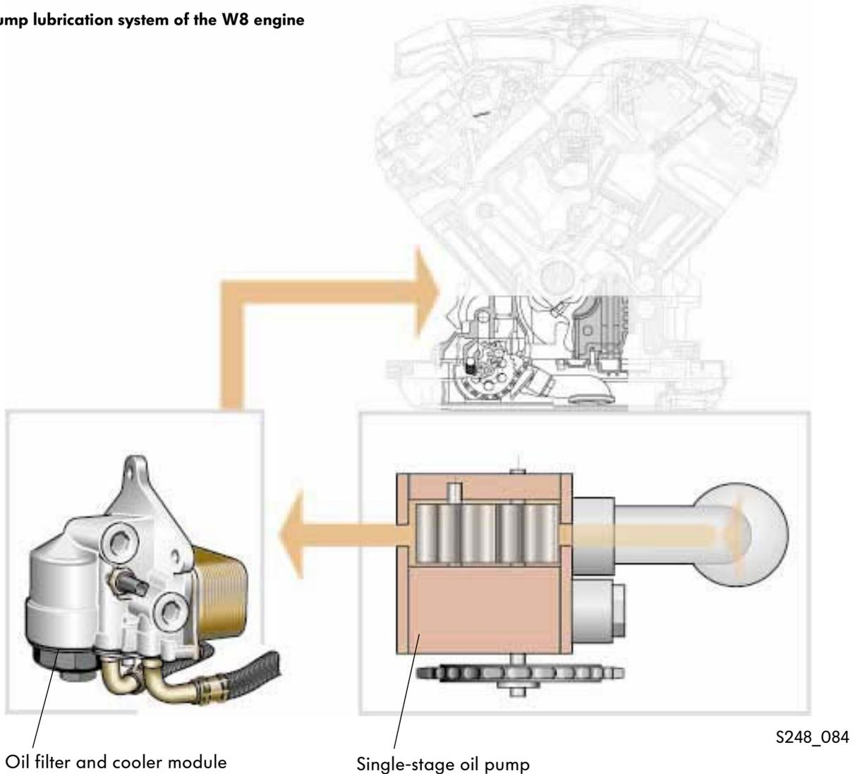
In the case of the wet-sump lubrication system, the entire oil supply is retained in the oil sump. The single-stage oil pump draws the oil out of the wet sump via the intake line and immediately returns it to the engine after it has cooled down and has been filtered.
