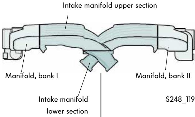
The intake manifold used in the W 12 engine is made of magnesium alloy. Unlike the W8 engine, each of the manifolds is coupled to a throttle valve control unit.
