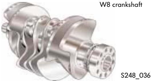
The crankshafts used in the W engines are manufactured from forged tempered steel. In each case, two conrods run between two main bearings.
