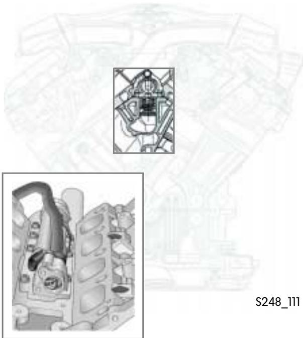
Switching over is affected by an electrically actuated thermostat valve. In the W8 and W12 engine, this valve is installed in the crankcase upper section from above. To replace this valve, it is necessary to remove the intake manifold.
