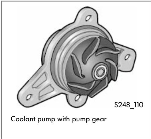
In both W engines, the coolant pump is located in the cylinder block at the face end. It is mounted directly upstream of the central coolant duct and is driven by the ribbed V-belt.
