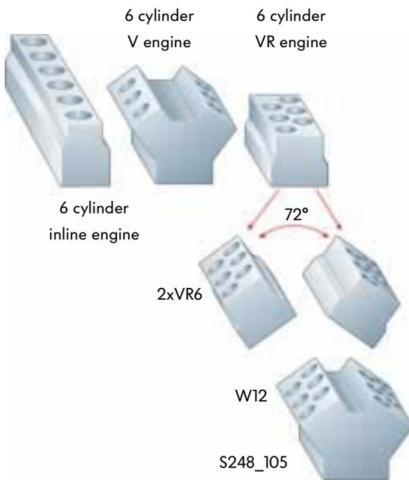
With regard to the evolution of the 6-cylinder engine, the VR6 engine stands out due to its compactness. It is much shorter than the comparable inline engine, and narrower than the V engine. Combining two VR6 engines with a cylinder angle of  $72^\circ$  produces a W12 engine.
