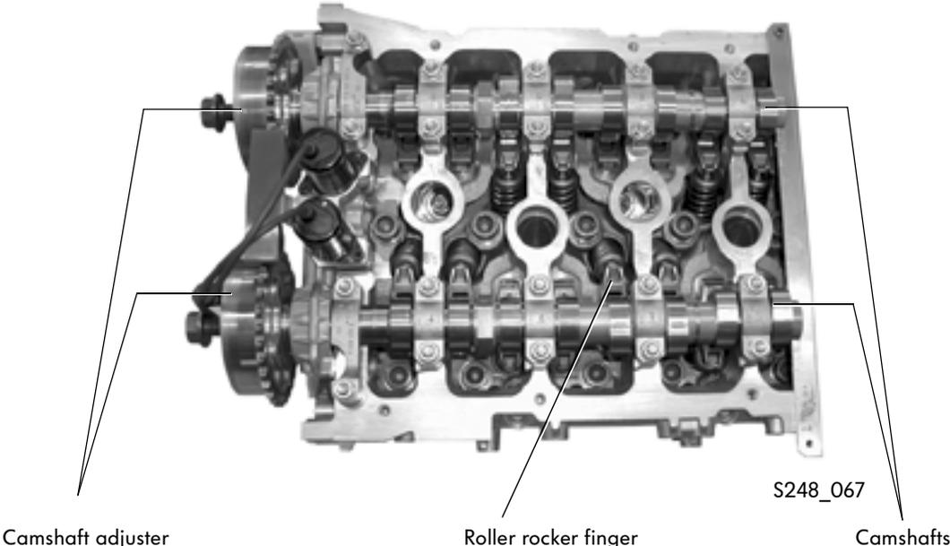
The 4 valves in each cylinder are actuated by low-friction roller rocker fingers. Valve clearance is compensated by hydraulic support elements.
