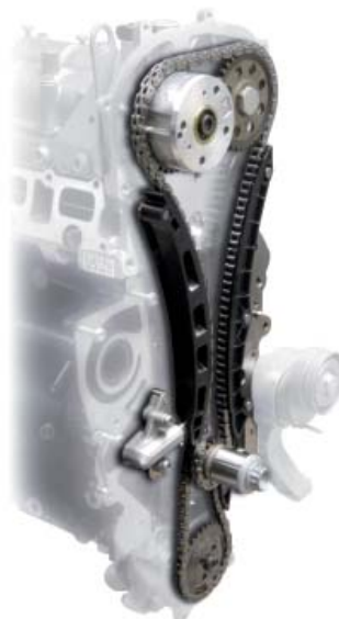
Maintenance-free chain drive (longlife)
