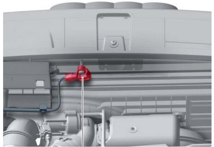
Front airbag crash sensor, driver side G283
