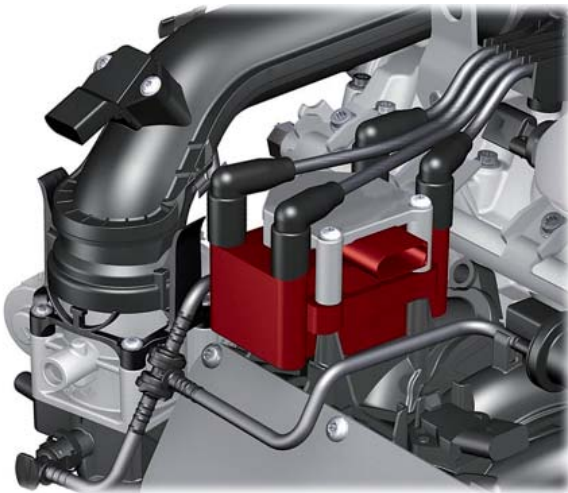
One ignition transformer for all four cylinders
