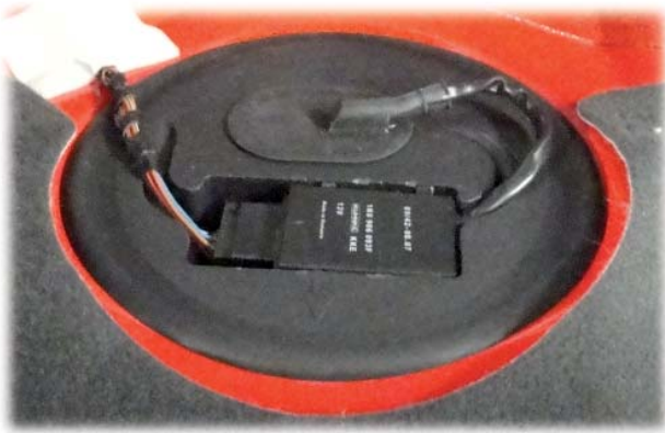
Demand-driven fuel system with fuel pump control unit
