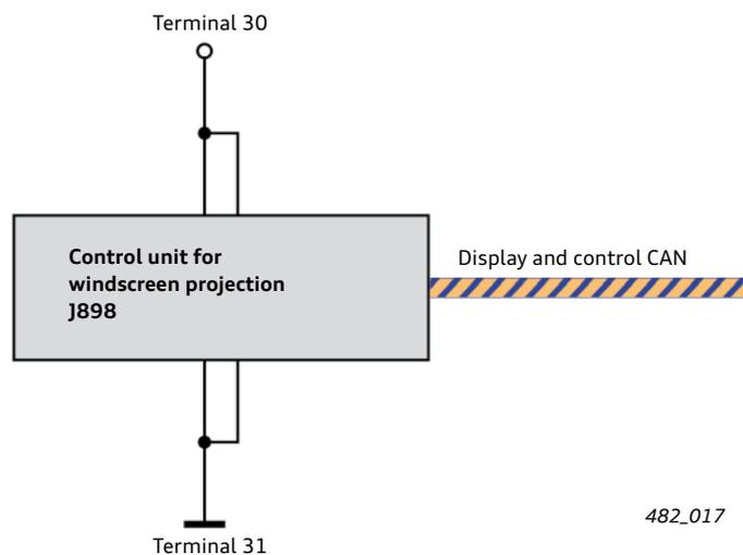
The control unit J898 receives information from the following control units for the head-up display:
