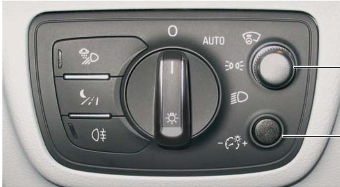
Position controller for head-up display (button for windscreen projection E736)
