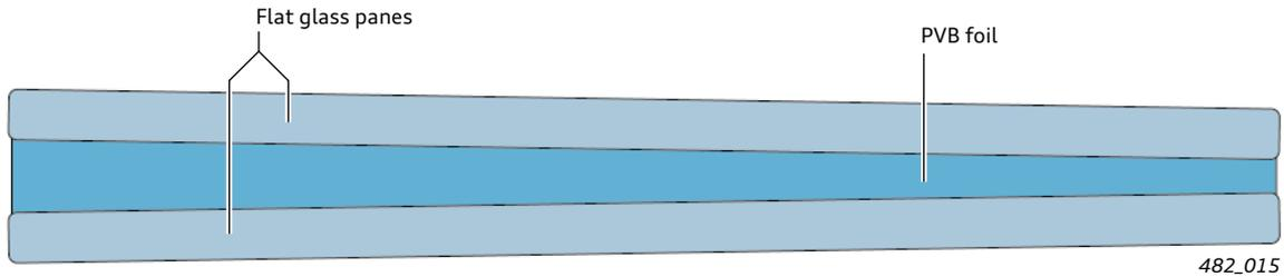
Windscreen in the case of a vehicle with head-up display
