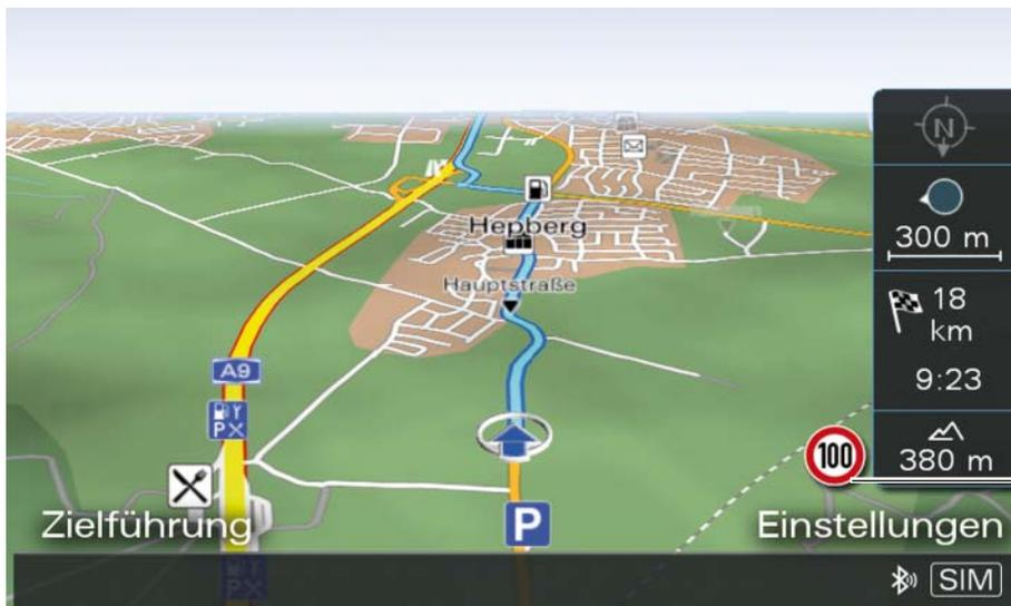
Representation of road signs with prescribed speeds in the speed limit indicator based on navigation data
