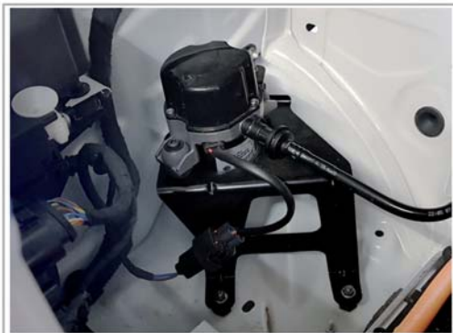
Vacuum pump V22 for brake booster in the motor compartment on the right
