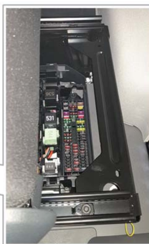
Under driver seat, relay carrier and fuse holder B (SB)
