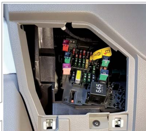
In the dash panel Relay carrier and fuse holder C (SC) with onboard supply control unit J519 and instruction flag
