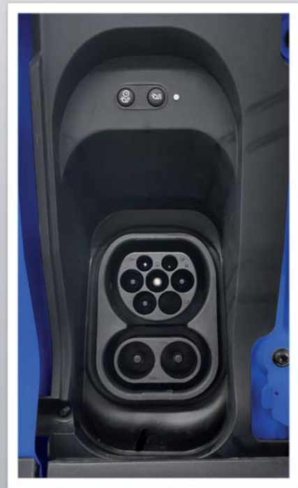
Charging socket behind the tank cap
