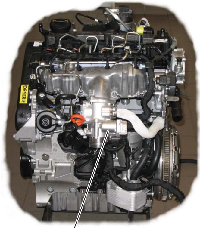
Throttle Valve Control Module J338 with Throttle Position (TP) Sensor G69
