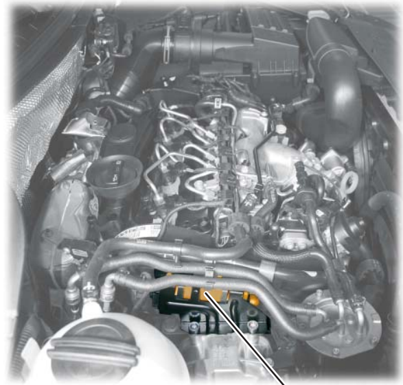
Auxiliary Fuel Pump V393
